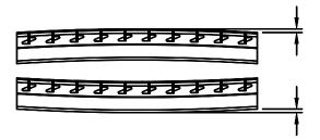
e. <u>Transverse Camber</u> = 0.004\*Width (in direction of cross bar or distribution bar).
