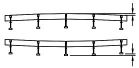
f. Sweep (side bow) = 0.025\*L (in feet) for panels up to 40'-0", inclusive, and 0.00065\*L<sup>2</sup>, for panels greater than 40'-0".
