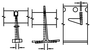
Note: No more than 1% of all locations can violate specified tolerance. No tolerance necessary for cross bars when encased in concrete on partial and full-depth grid systems.
