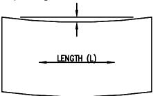
Note: Sweep tolerances applicable for galvanized panels with standard puddle welds connecting components and diagonal grids less than 25' in length. Galvanized diagonal open grid panels not recommended over 25' in length.
