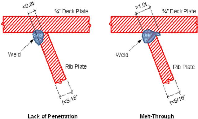
Figure 4: Defects in Rib-to-Deck Partial Joint Penetration (PJP) Welds
