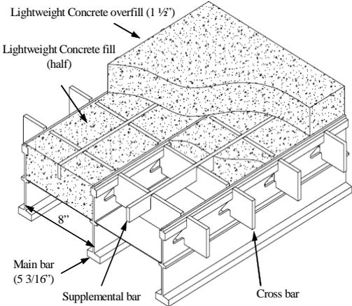
Figure 5: Details of New Grid Deck
