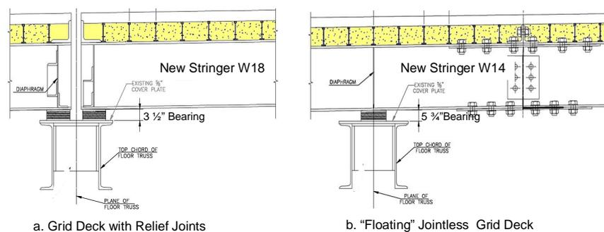
Figure 6: Both Deck Options and Their Elastomeric Bearings
