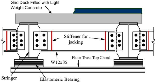
Figure 7: New Grid Deck, Stringers, and Elastomeric Bearings
