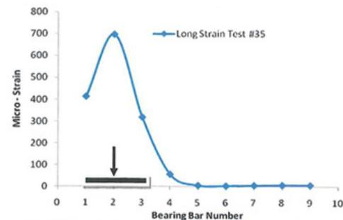
Figure 1: Results are from test on 37R5 Lite 5" x 1/4" riveted steel deck. Maximum response is from the three bearing bars directly under the simulated tire patch. Main bars are spaced at 5.125" on center.
