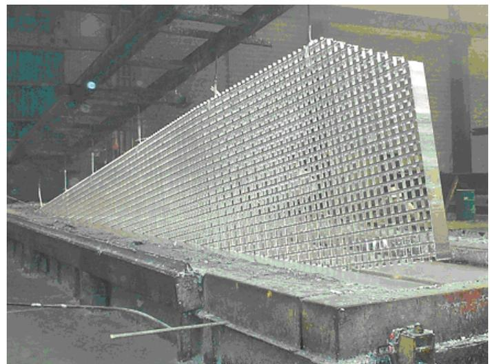
*Hot-Dip Galvanized Grid Deck Panel*
